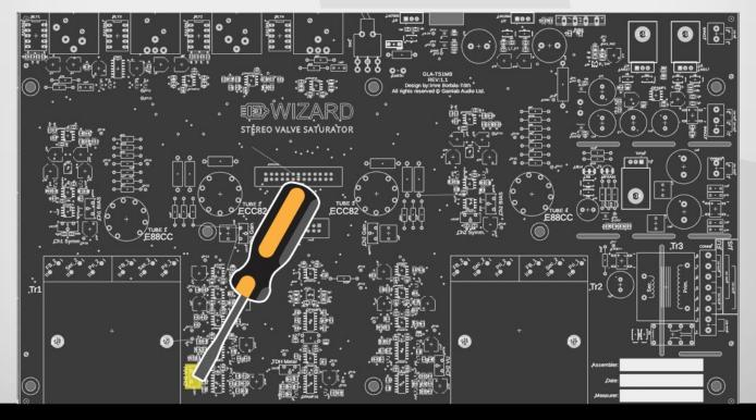
APPLY A 0dBu, 1 KHZ SINE SIGNAL TO THE INPUTS. MEASURE THE OUTPUT LEVEL, AND SET THE INPUT AND OUTPUT POTENTIOMETERS AROUND THE 0dB POSITION SO THAT THE OUTPUT READS EXACTLY 0dBu. THEN TURN THE CH2 VU TRIMMER CLOCKWISE UNTIL THE R LED METER ON THE UNIT INDICATES -3dBu. NEXT, SLOWLY TURN THE TRIMMER COUNTERCLOCKWISE UNTIL THE 0dBu LED LIGHTS UP.
