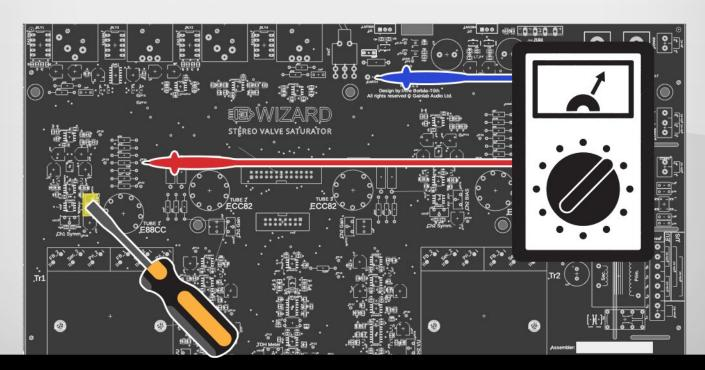
MEASURE THE **DC VOLTAGE** BETWEEN **TP19** AND **TP20**, AND **ADJUST THE CH1 SYMM TRIMMER** TO ACHIEVE THE VALUE **CLOSEST TO 0V**. *IF THE MEASURED VALUE EXCEEDS* **100MV**, THE TUBE IS EITHER WORN OUT OR DEFECTIVE. REPLACE THE TUBE!
