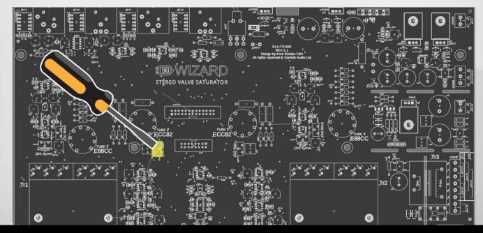
TURN BOTH THE INPUT AND OUTPUT POTENTIOMETERS FULLY CLOCKWISE. APPLY A -20dBu, 1 KHZ SINE WAVE TO THE INPUT. MEASURE THE OUTPUT USING A BALANCED-INPUT INSTRUMENT OR AUDIO INTERFACE. ADJUST THE CH2 GAIN TRIMMER UNTIL YOU MEASURE A +14dBu OUTPUT SIGNAL.
