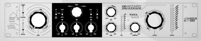
APPLY A +12dBu, 1KHZ SINE SIGNAL TO THE INPUT. WHILE MONITORING THE OUTPUT OF CH1 OR CH2, MEASURE THE DISTORTION (THD). SLOWLY INCREASE THE INPUT POTENTIOMETER UNTIL THE OUTPUT SHOWS APPROXIMATELY 5% THD ON AN EXTERAL THD METER. THEN USE THE THD METER TRIMMER TO ADJUST THE FRONT PANEL INDICATOR SO THAT IT DISPLAYS 5% THD. AFTERWARDS, VARY THE INPUT POTENTIOMETER AND OBSERVE WHETHER THE DISTORTION LEVELS FOLLOW THE LED INDICATOR CONSISTENTLY.
