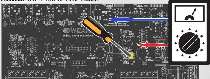
MEASURE THE DC VOLTAGE BETWEEN **TP26** AND **TP27**, AND ADJUST THE **CH2 SYMM TRIMMER** TO ACHIEVE THE VALUE CLOSEST TO **0V**. *IF THE MEASURED VALUE EXCEEDS* **100mV**, THE TUBE IS EITHER WORN OUT OR DEFECTIVE. REPLACE THE TUBE!
